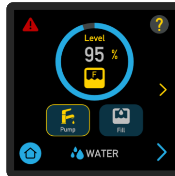
Water tank monitoring and pump controls
